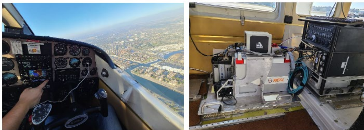
Fig. 2.7 Aircraft-mounted Modular Aerial Sensing System used to survey the Eaton and Palisades fire areas. Instruments consist of IMU, LiDAR, and IR, Hyperspectral, and RGB cameras.
