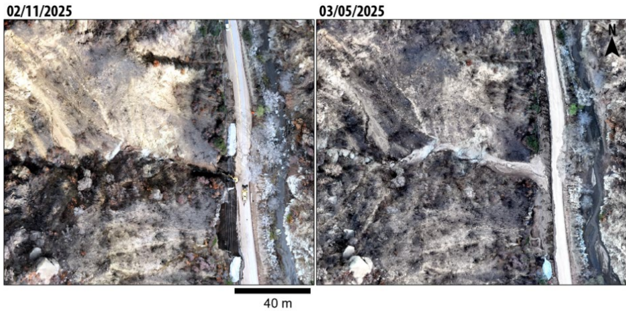
Fig. 2.19. Drone optical image comparison before and after the Feb 13 storm. The debris flood/flow deposits near the State Route 27 road are shown in Figure 2.17.
