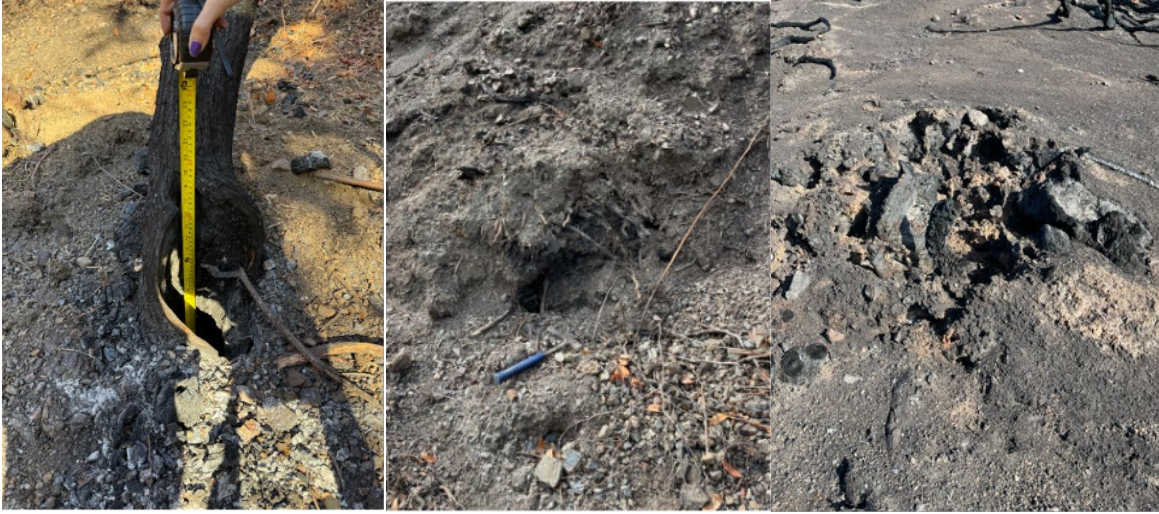
Fig. 2.12. Macropores due to combusted roots (coordinates: 34.120597°, -118.506639°; 34.117769°, -118.505200°; 34.046954°, -118.559453°)
