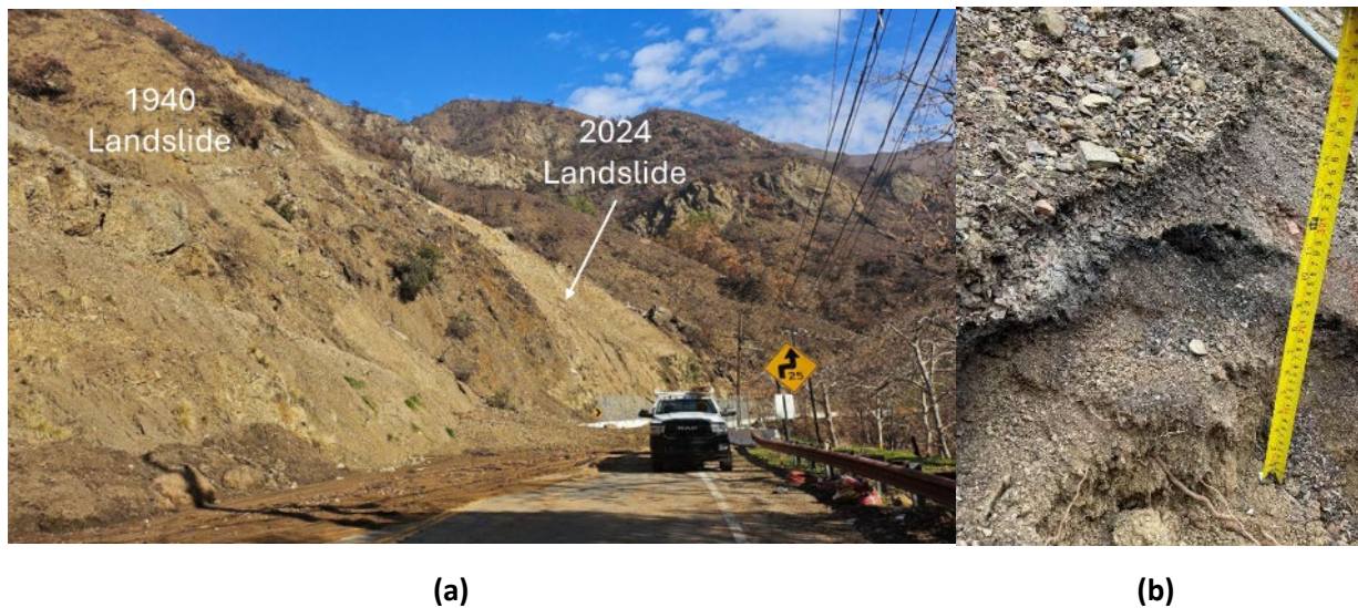
Fig. 2.32. (a) Mud and debris blocking State Route 27 after the February 13, 2025 storm. (b) Debris covering the ash layer in the 1940 landslide area (coordinates: 34.063016°, -118.585803°; 34.063365°, -118.586363°).
