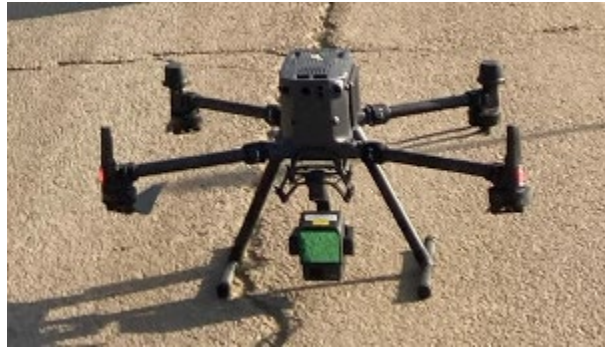
Fig. 2.5. Unpiloted aerial vehicle carrying a lidar sensor system used for high-resolution post-fire topographic mapping.
